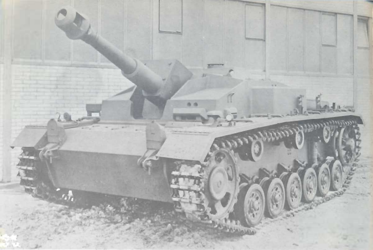
The "Sturmhaubitze 42" as Ausfuehrung F. The vehicle is identical to the "Sturmgeschuetz 40", but mounts the 10.5 cm gun.
