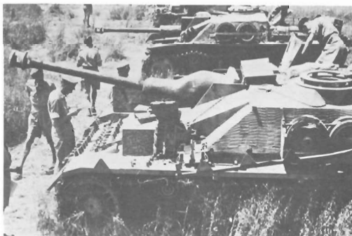
A good superstructure comparison between both "Sturmgeschuetz" types. The longer "Panzer IV" chassis asked for modifications to the regular assault gun fighting compartment. "Sturmgeschuetz IV" is in foreground.
