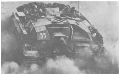
Noticeable here are the drive and idler sprockets and the original spacing of the return rollers. The box-like protrusion on the left side of the superstructure housed radio equipment.
