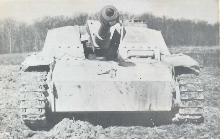
Front and rear view of "Sturmhaubitze 42" demonstrate the compact, low silhouette of the vehicle.
