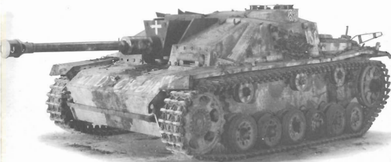
Owing to the severe raw material shortage in Germany during 1944 and 1945, some of the return rollers for assault guns were supplied without the usual rubber tires. This vehicle is covered with a "Zimmerit" protective coat to eliminate magnetic anti-tank mines. Also seen is the bullet-splash proofing of the cupola, which appeared on late-production models. It is obvious that some of the front torsion bars on this vehicle are broken.
