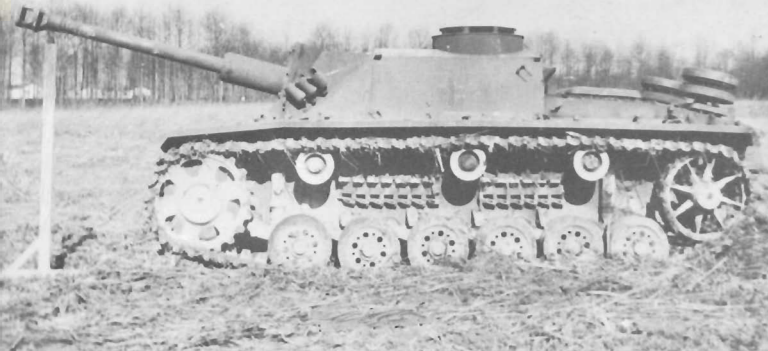
Besides armor skirting, quite common on "Sturmgeschuetz" vehicles, additional protection was achieved by attaching spare track links to both hull sides, where only 30 mm base armor was provided.
