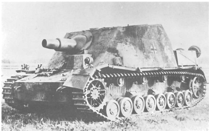
This "Sturmpanzer 43", built only in limited numbers, appeared with two different driver compartment configurations. The unchanged Panzer IV chassis was used.
