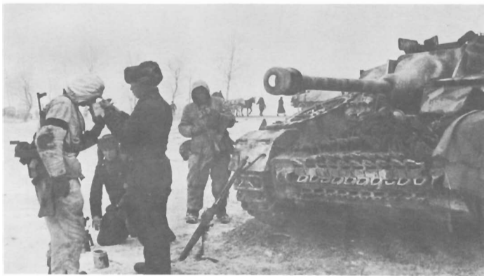
Assault gun IV in Russia. One of the recognition features was the box-like driver compartment. Note extra drive sprocket stowed away on vehicle.
