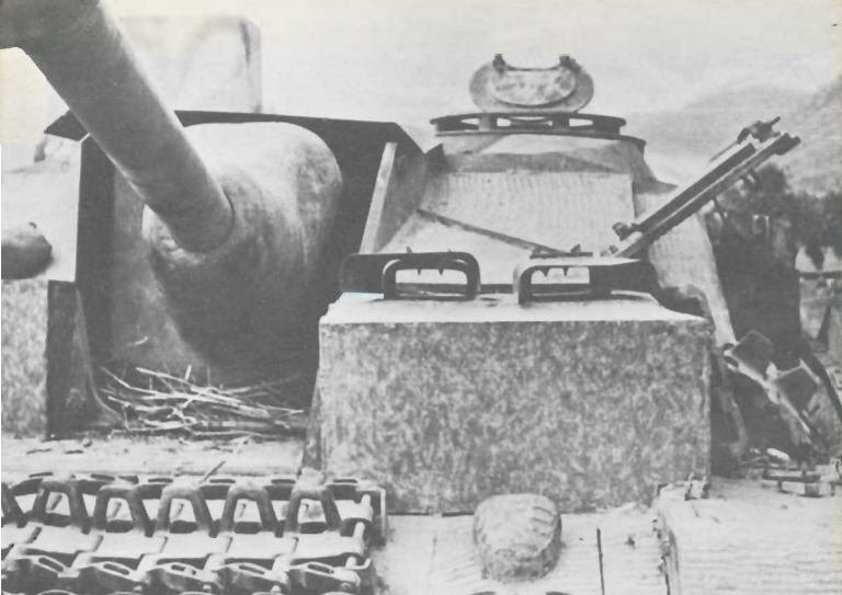
A close-up view of the driver compartment with vision episcopes and hatch cover. The cast gun mantlet can clearly be seen in all details.
