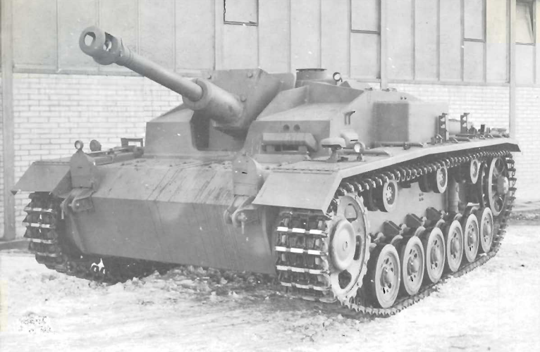
This factory picture shows the first production model of the "Sturmgeschuetz III" mounting the long 75 mm StuK 40 L/43. Called Ausf. F, it also offered a ventilated fighting compartment and other minor modifications to the superstructure.
