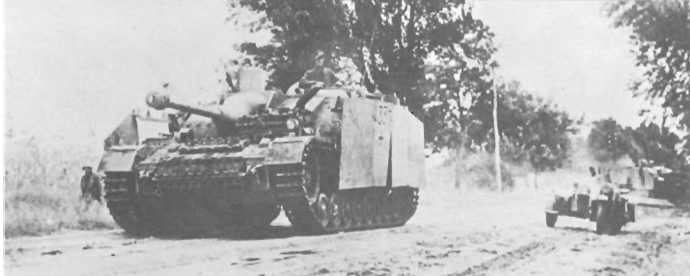
The "Sturmgeschuetz IV" was very similar to the "Sturmgeschuetz III". "Saufkopf" mantlet and bolted-on frontal armor, together with armor skirts, made identification sometimes difficult.
