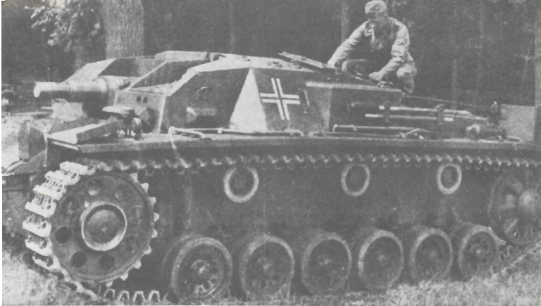
Noticeable here are the drive and idler sprockets and the original spacing of the return rollers. The box-like protrusion on the left side of the superstructure housed radio equipment.
