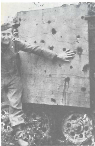
The effect of Russian anti-tank rifles, against the skirt armor of a "Sturmgeschütz". An inexpensive and effective protection against small arm fire to protect the weak armored flanks of these vehicles.
