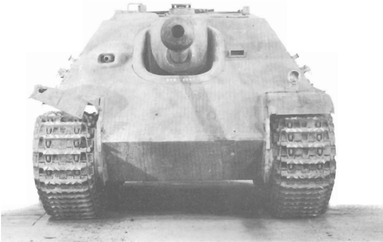
Frontal view of this tank-destroyer indicates the pronounced slope of the front plate, the ball mount for the radio operator MG and the vision slit for the driver.
