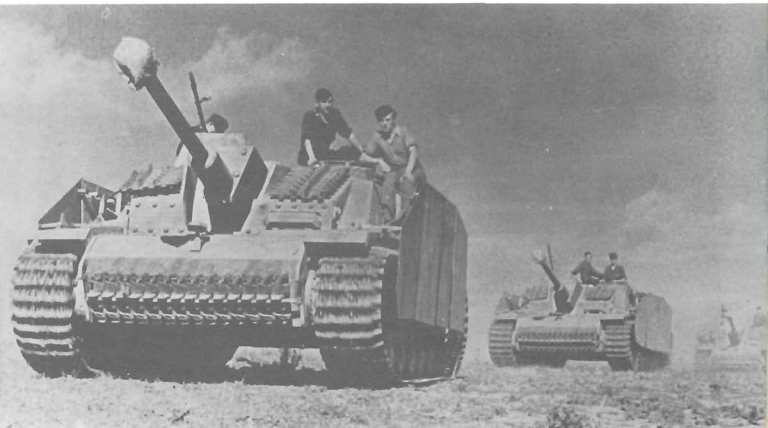
"Sturmgeschuetze" in Russia, 1944. Standard armor skirt protection can be seen, as well as the attachment of additional track links to provide extra resistance against the very effective Russian anti-tank rifle.
